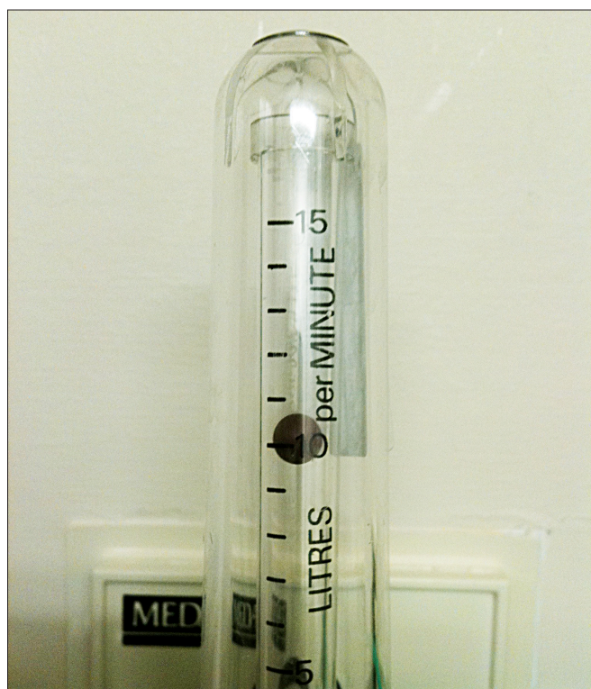
Figure 4. Oxygen flow meter. Read off flow rate from the centre of the plastic ball e.g. this valve is supplying 10L/min.
