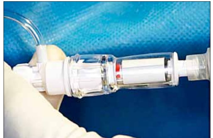
Figure 7: The indicator within the hub of the SafeTcentesis (UK Medical, Sheffield, UK) turns from red to white when the pleura is breached.
